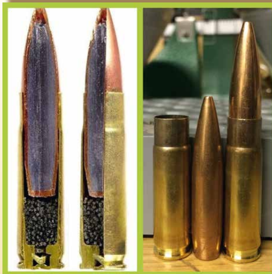
Slika 2: Tulec in naboj .300 AAC Blackout, prerez
