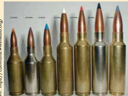
Slika 2: WSM in WSSM naboji: .223 WSSM, .243 WSSM, .25 WSSM, .270 WSM, 7 mm WSM, .300 WSM, .325 WSM
