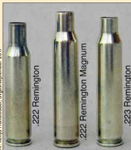
Slika 1: Primerjava tulcev kalibrov .222 Remington, .222 Remington Magnum in .223 Remington
