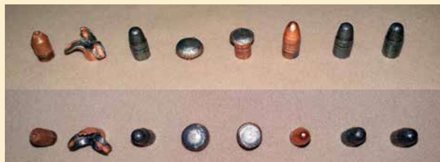
Deformacija krogel po zadetku v želatino (z leve proti desni si sledijo: CCI Copper-22, CCI Quiet Segmented HP, CCI Quiet RN, CCI Stinger, CCI Velocitor, Federal Suppressor, CCI Standard Velocity, Lapua SK Standard).
