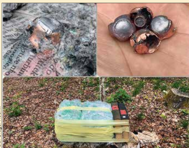
Sl. 6: Testiranje preoblikovanja krogel BallisticTip Hunting in Partition
